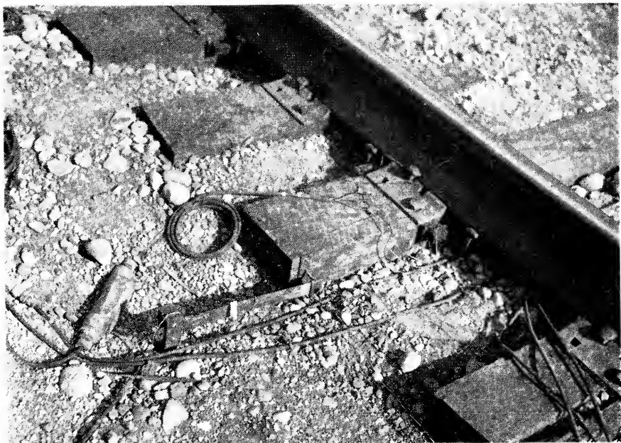
Fig. 4. Deflectometer for Measurement of Tie Movement in the Ballast
